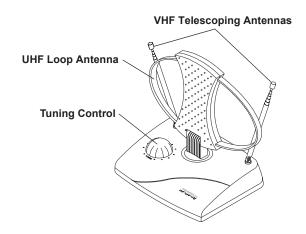
Fully extend the telescoping antennas for viewing VHF-Lo TV Channels 2–6 in Canada.
